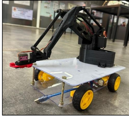
Fig.11 Isometric view of Pick and place robot
