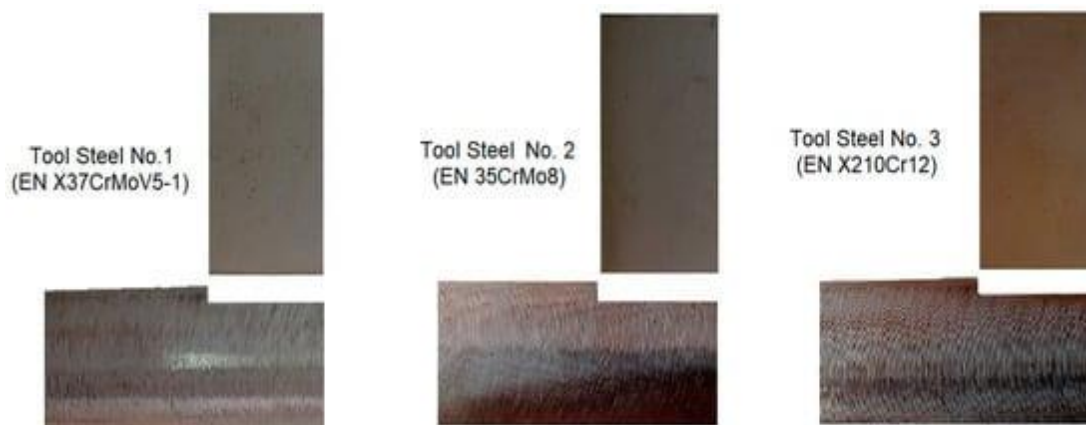
Fig.4.1.WEDM-produced experimental samples of tool steels EN X37CrMoV5-1, EN 35CrMo8, and EN X210Cr12 at the L1 level of the MTP parameters.
