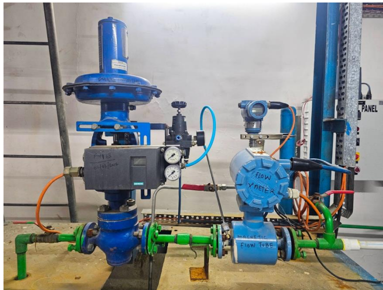
Fig. 1 Experimental Setup of Flow Control System.
