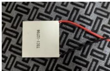
Figure 1. The thermoelectric module used in the experiment, TEC1-12706.
