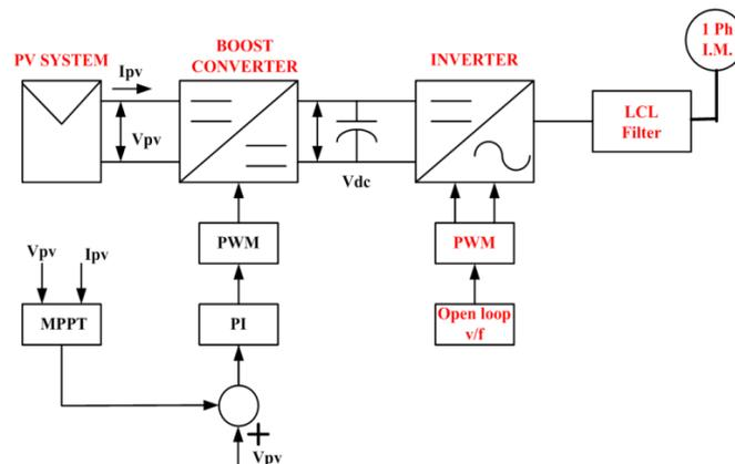
**Figure 3 Control block diagram of islanded mode**
