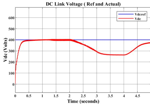
**Figure 12 DC link voltage in islanded mode**
