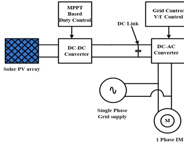
**Figure 1 Reduced converter topology for Solar Water Pump System**
