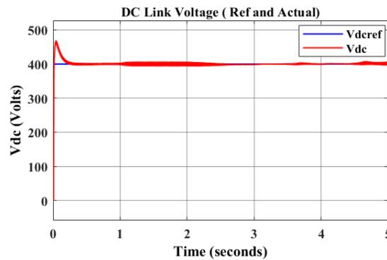
**Figure 7 DC link voltage in grid connected mode**
