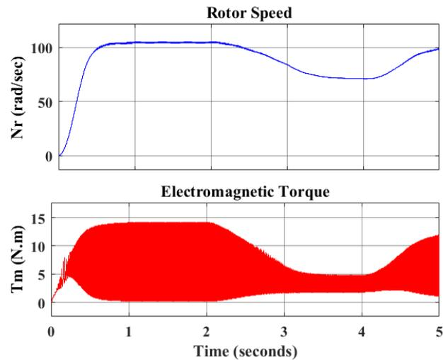
**Figure 14 Motor speed and torque in islaned mode**
