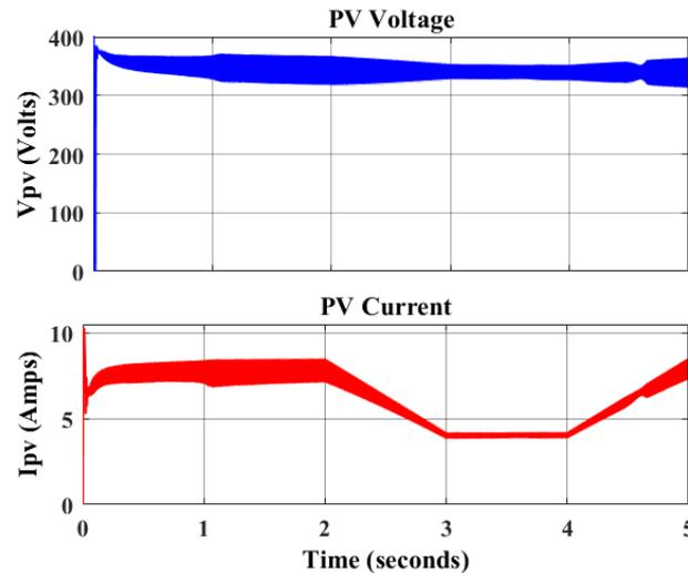
**Figure 4 PV voltage and current in grid connected mode**
