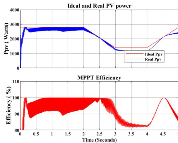
**Figure 11 Ideal and real PV power and its efficiency in islanded mode**
