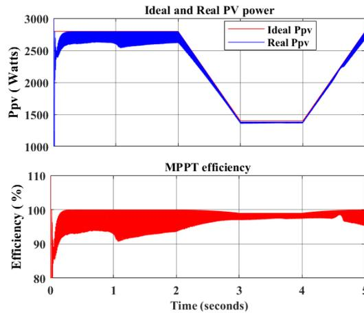
**Figure 6 Ideal and real PV power and its efficiency in grid connected mode**
