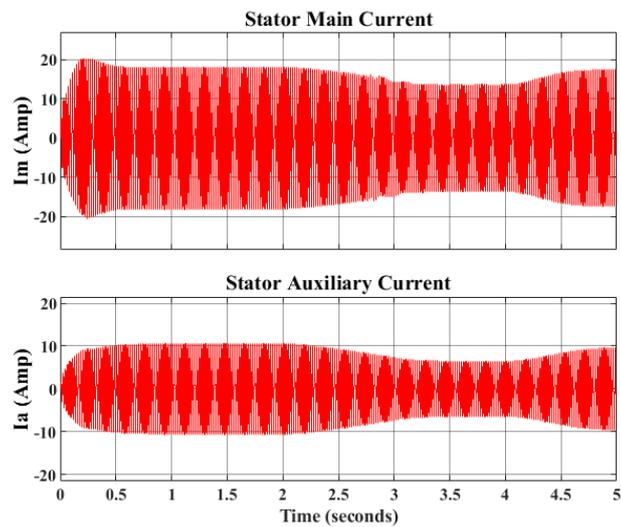
**Figure 15 Motor main and auxiliary current in islaned mode**
