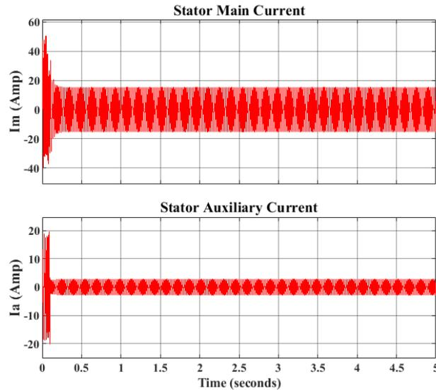
**Figure 9 Motor main and auxiliary current in grid connected mode**
