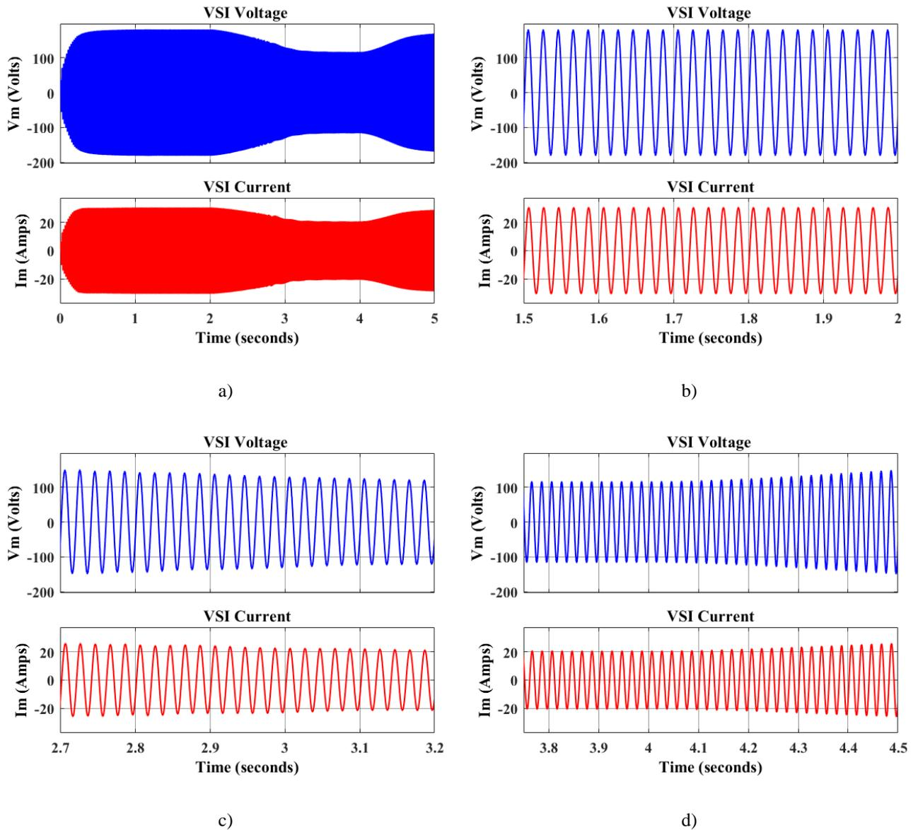
Figure 13 VSI Voltage and Current in islanded mode
