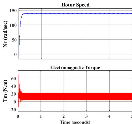
**Figure 8 Motor speed and torque in grid connected mode**
