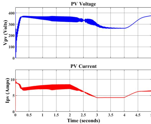
**Figure 10 PV voltage and current in islanded mode**
