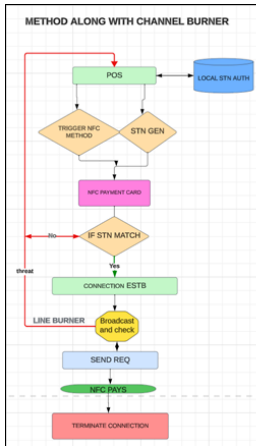
Figure 4 System Architecture for proposed solution
