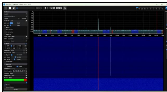
Figure.1 Default configuration for NFC signals
