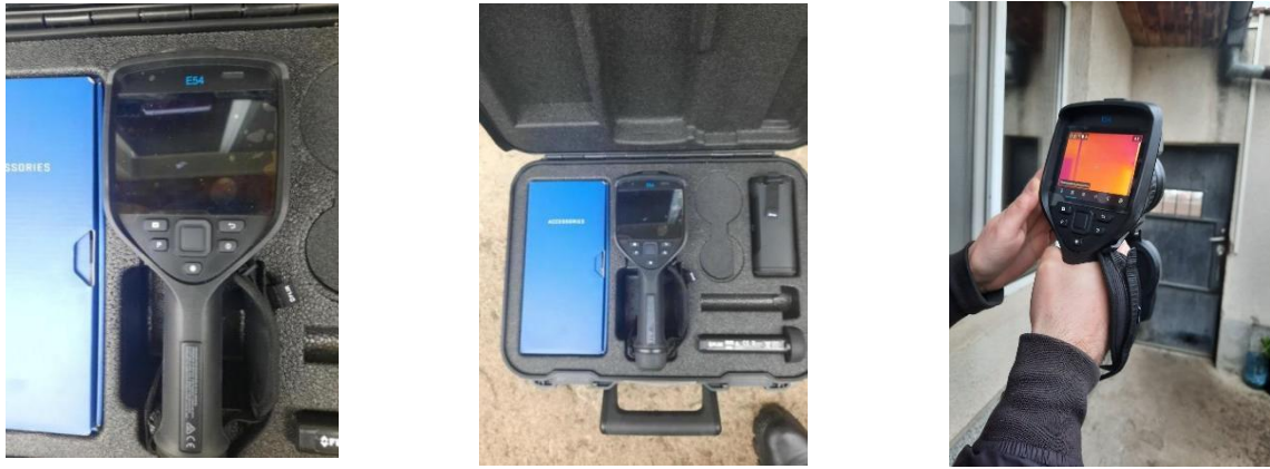
Fig. 2 Thermal camera E54 for thermal inspection of livestock farm buildings with a controlled microclimate
