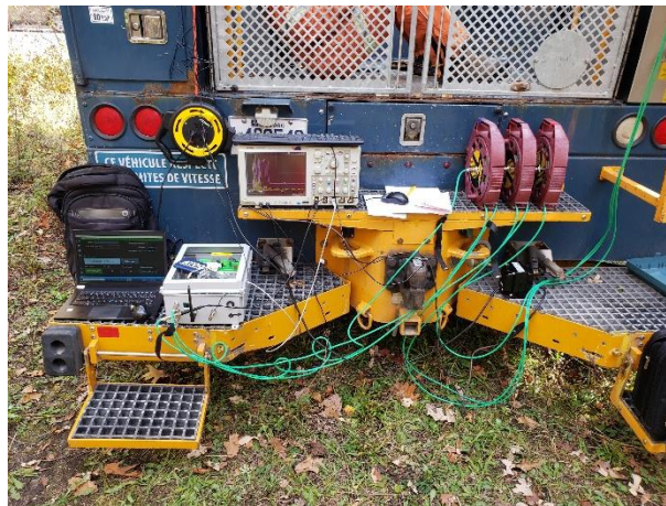
Fig. 12 Detection unit UD 2 (IED and green sensor cables), oscilloscope and portable computer
