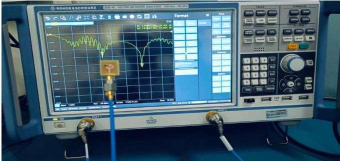
Fig. 7. Measured Return Loss of the Proposed Antenna when Diode is OFF
