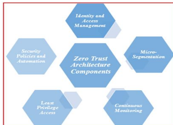
Figure 1: Zero Trust Architecture Components
