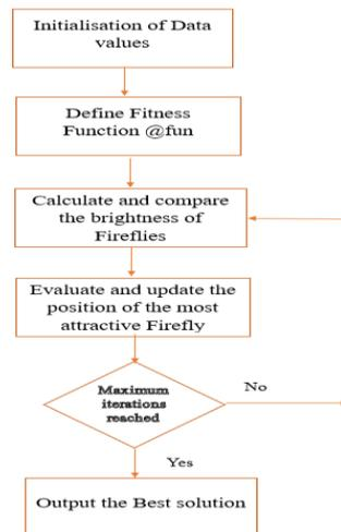
**Figure 3.** Flow chart of Firefly Optimization Algorithm
