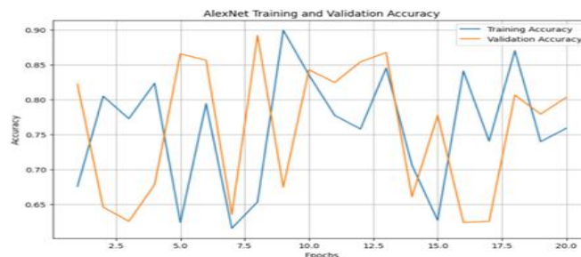
Fig 13 Training and validation accuracy of AlexNet Model
