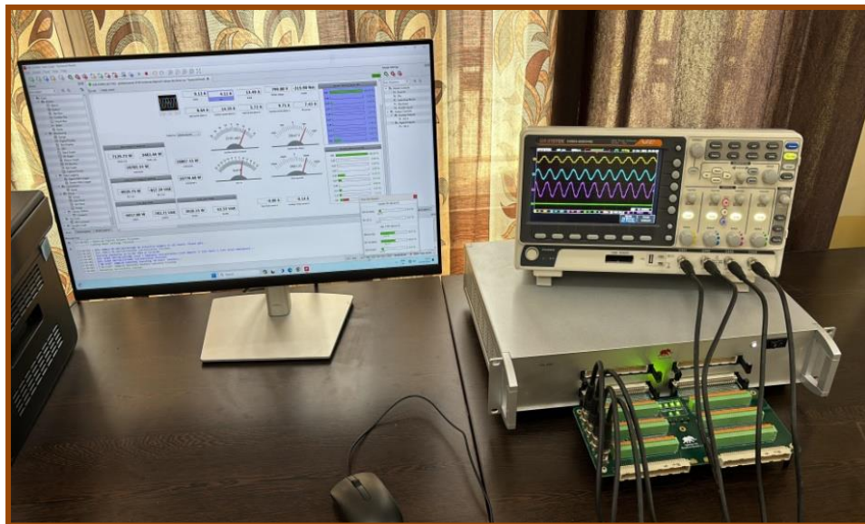
Fig. 3. Typhoon HIL 604 based real-time simulation setup.
