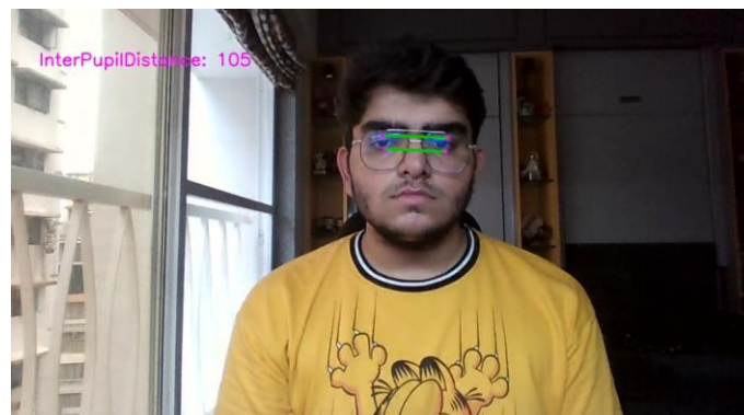
Fig.4: Inter-pupil distance feature extraction, using landmarks at the center top and bottom of each eye to accurately measure the distance.
