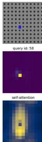
Figure 10: Decoder's query number and encoder's self-attention for detected defects in contact hole pattern
