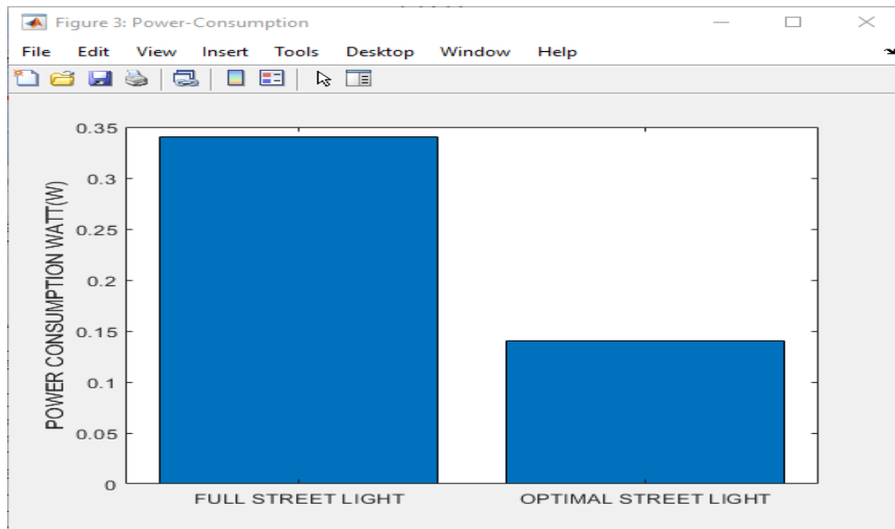
Figure 7: Power consumption for street intervals 6 and number of lights ahead 5
