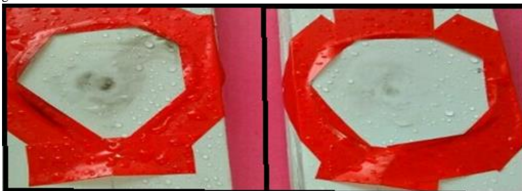
Fig. 8 Hydrophobicity check after HV test
