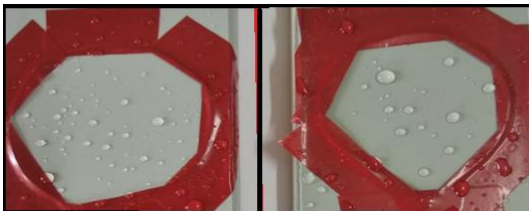
Fig. 7 Hydrophobicity check before HV test
