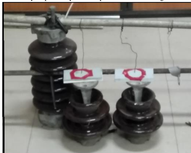
Fig. 6 Hydrophobicity test setup
