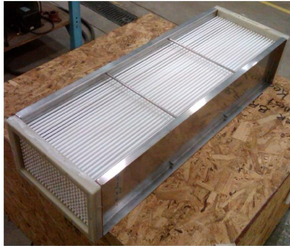
Fig.8. An example of a long TMC module designed and built for use in power plant boilers [33].
