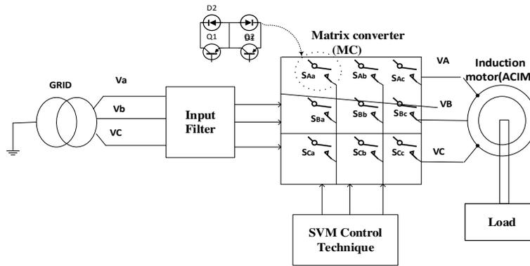
Figure.1: Block Diagram of DMC-IM
