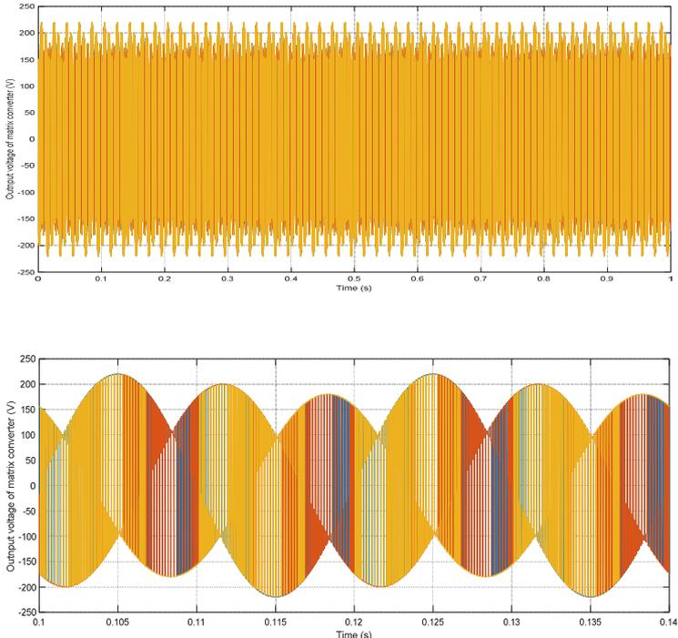
Figure. 14. Output voltages of matrix converter
