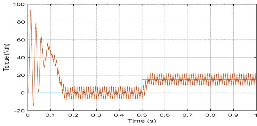
Figure. 16. Electromagnetic torque and reference.
