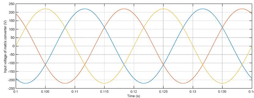
Figure. 6. Input voltage of matrix converter
