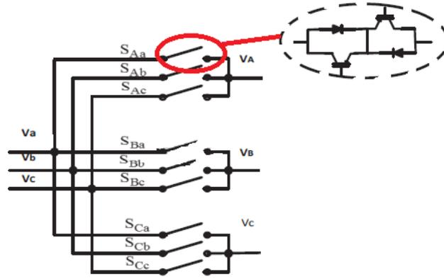
Fig. 2. Matrix converter structure.
