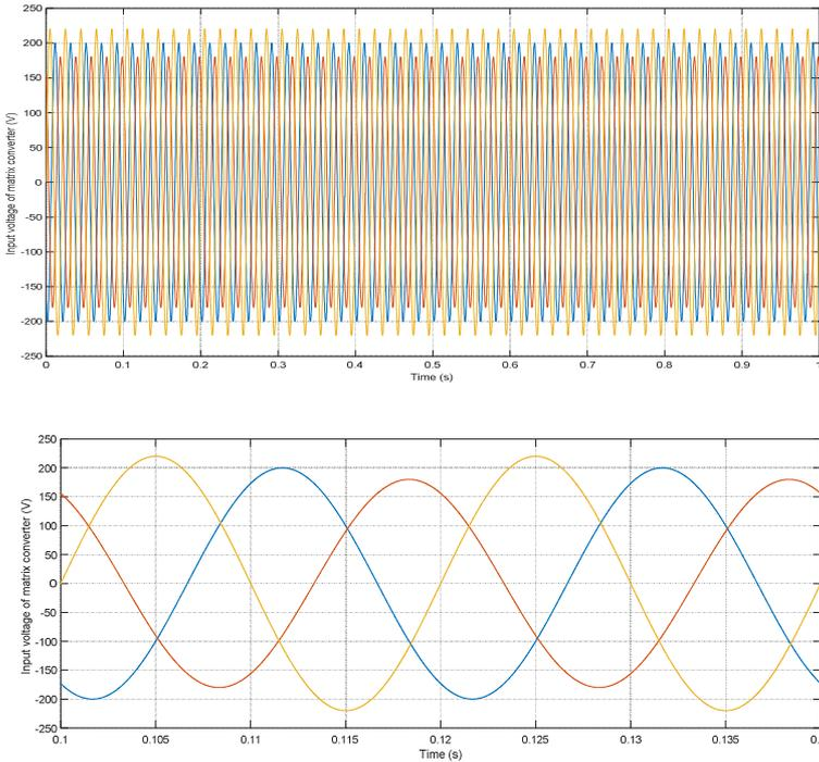
Figure. 13. Input voltages of matrix converter
