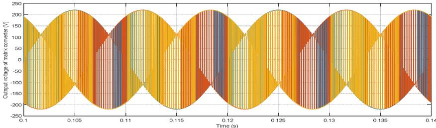
Figure. 8. Output voltage of matrix converter
