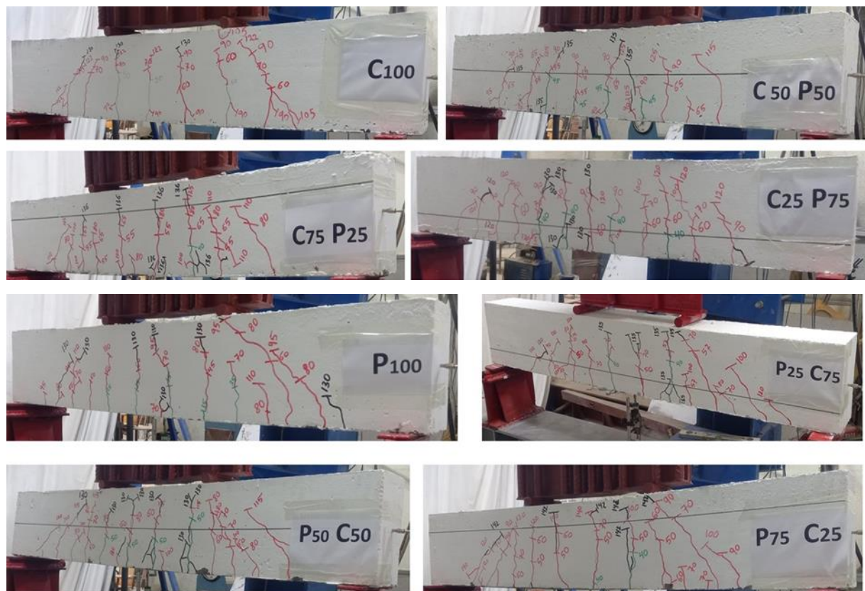
Figure 5. Cracking pattern of reinforced concrete beam laboratory samples.
