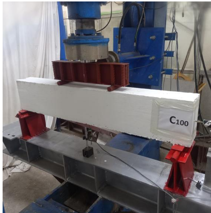
Figure 4. Reinforced concrete beam laboratory setup.
