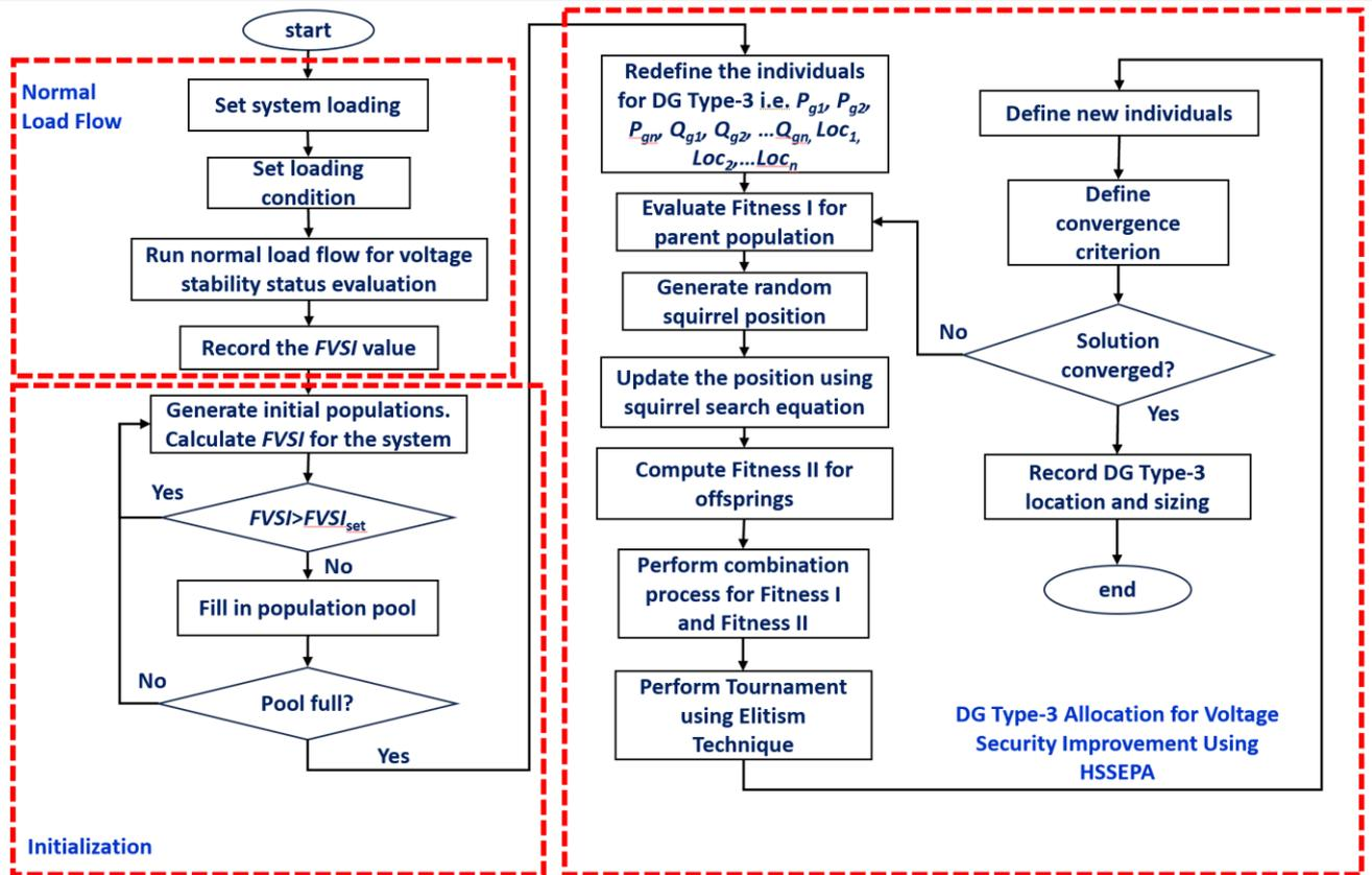
Figure 3: Proposed HSSEPA Technique for DG Type-3 Allocation in Voltage Security Improvement
