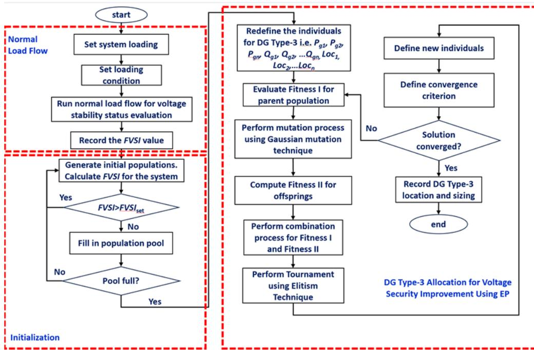
Figure 2: EP Technique Flowchart for DG Type-3 Allocation in Voltage Security Improvement
