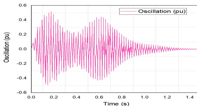
**Figure 4 (b).** Waveform of the torsional interaction for wind speed 8 m/s and 55% compensation with proposed controller of STATCOM
