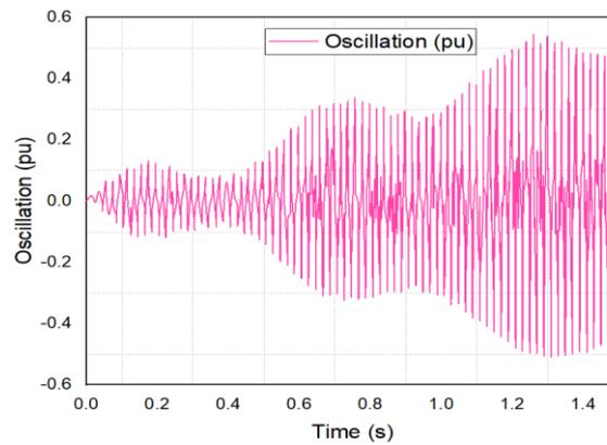
**Figure 4 (a).** waveform of the torsional interaction for wind speed 8 m/s and 55% compensation with conventional controller of STATCOM
