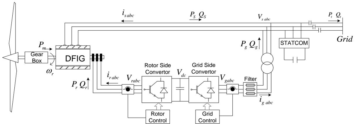
Figure 1. Strategy of STATCOM connected to DFIG
