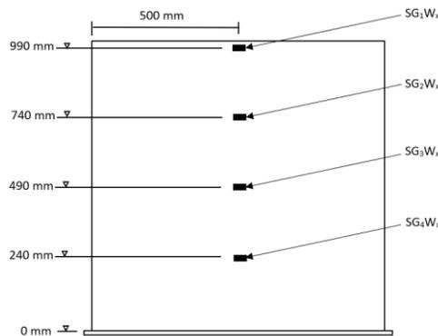
**Figure 3.** Strain gauges position (Side view).
