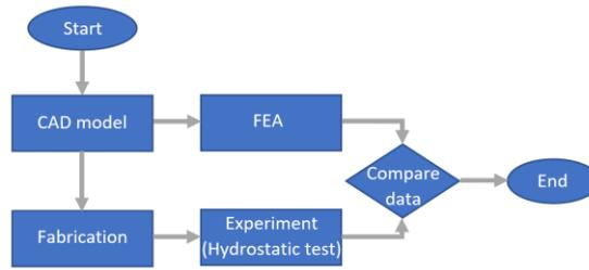
**Figure 1.** Stress comparison flowchart.
