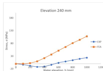
**Figure 9.** Stress comparison at el. 240 mm.
