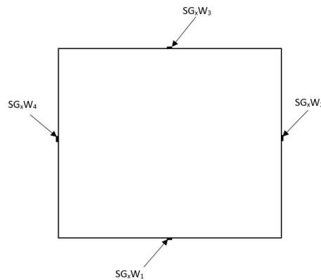
**Figure 2.** Strain gauges position (Plan view).
