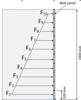
**Figure 4.** Load applied in FEM.
