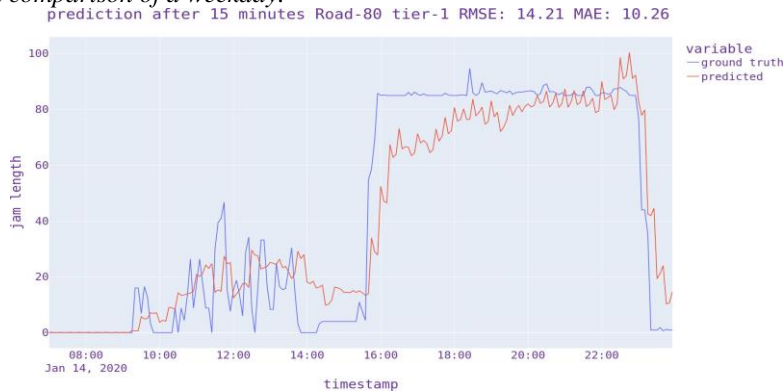
Figure 8. Prediction result based on USTGCN of road number 80 on one of the weekday of January,2020. (Training set: November 2019, December 2019). Here, tier-1 means road number 80 belongs to cluster number 2. But in USTGCN the clustering was not performed
