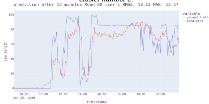
Figure 4. Prediction result based on USTGCN of road number 80 on one of the weekends of January,2020. (Training set: November 2019, December 2019). Here, tier-1 means road number 80 belongs to cluster number 2.
