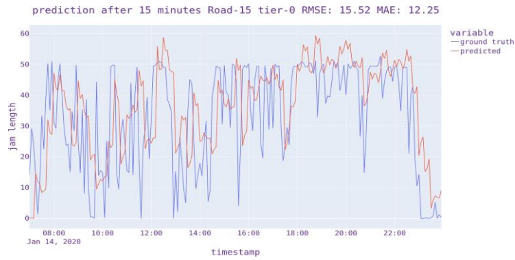
Figure 6. Prediction result based on USTGCN of road number 15 on a weekday of January,2020. (Training set: November 2019, December 2019). Here, tier- 0 means road number 15 belongs to cluster number 1. But in USTGCN the clustering was not performed
