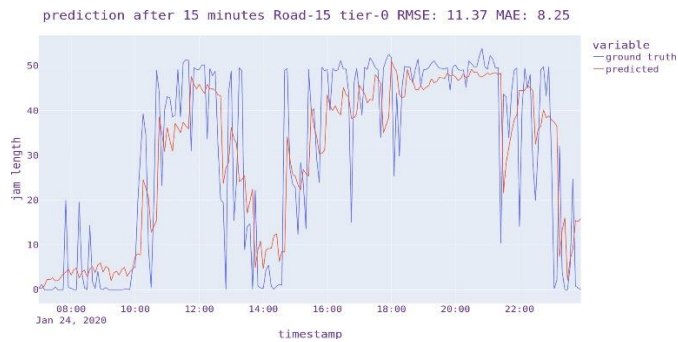
Figure 1. Prediction result based on modified USTGCN (2 clusters) of road number 15 on one of the weekends of January,2020. (Training set: November 2019, December 2019). Here, tier-0 means road number 15 belongs to cluster number 1
