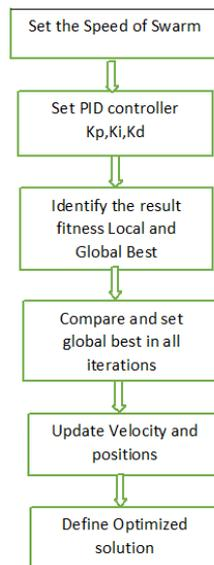
Fig. 2 Flow chart of step for PSO-PID optimization
