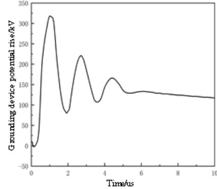
Fig. 7. The grounding device potential rises (0m in seawater layer)
