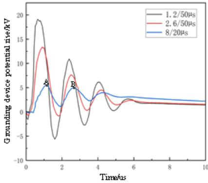
Fig. 11. Grounding potential rise under different lightning current waveforms (10m in seawater layer)
