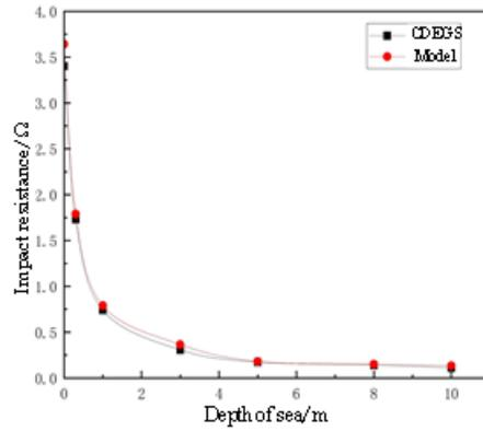
Fig. 8. Effect of seawater depth on impulse resistance
