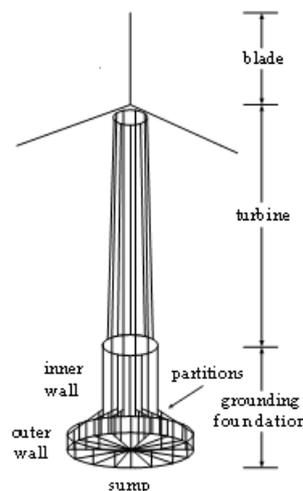
Fig. 3. Wind turbine overall model diagram
