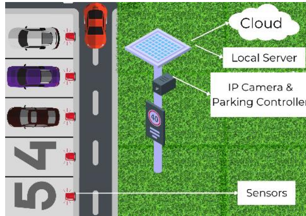
Fig. 4. IoT System of Car Parking
