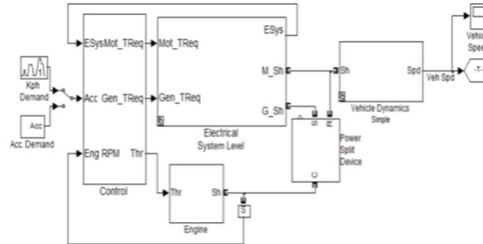
Figure 6: Block diagram of Energy Management Systems
