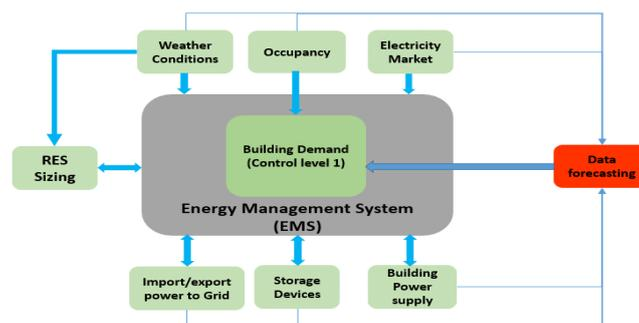
Figure 7: Block diagram of Energy Management Systems
