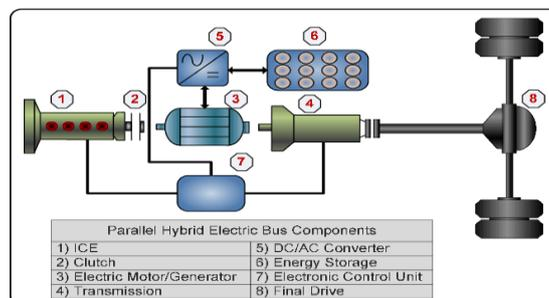
Figure 1: Common hybrid-electric vehicle architectures Parallel
