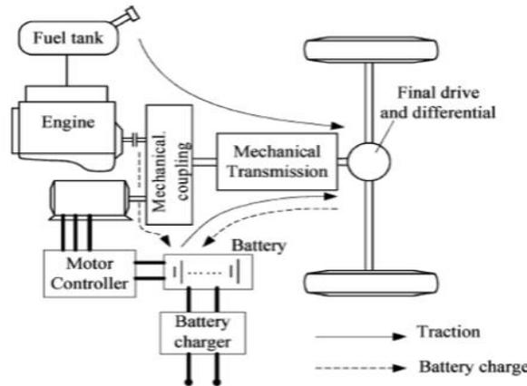
**Figure 3: Block diagram of parallel configuration of HEV**
