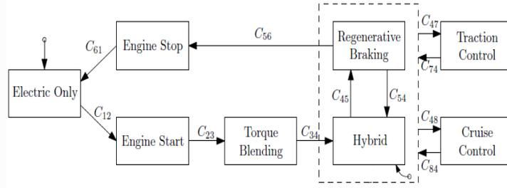
**Figure 5: A state machine representation of the vehicle supervisory controller.**
