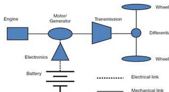
Figure 2: Schematic of parallel hybrid power train configuration.
