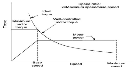
Figure 8: Motor ideal torque-speed characteristics.
