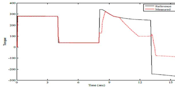
(b) Motor torque- characteristics.
