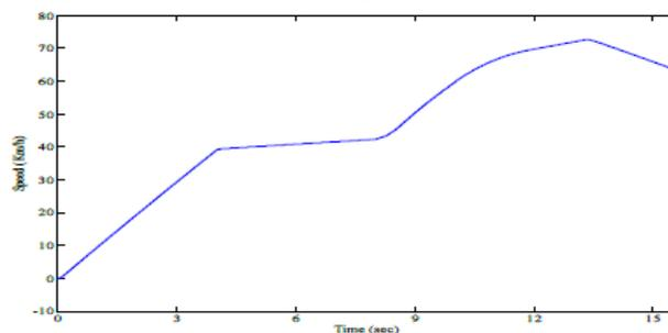
(a) Motor speed characteristics.
