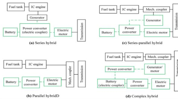
**Figure 4: A comprehensive review on hybrid electric vehicles: architectures and components**
