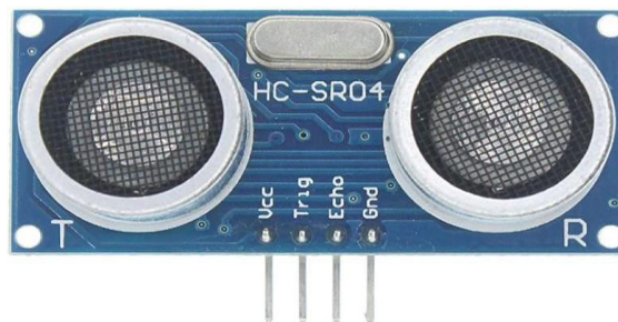
Fig. 2 Ultrasonic Wave Sensors (the HC-SR04 ultrasonic sensor)
