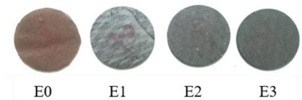
FIG. (1): THE SAMPLES FOR THERMAL CONDUCTIVITY TEST.
