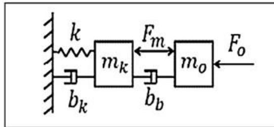
Fig.4 Series elastic actuator model with applied load.[25]
