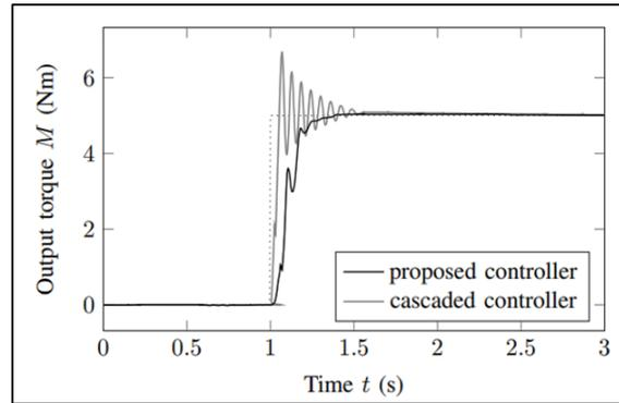
Fig.12 Step response of the closed loop system [30]
