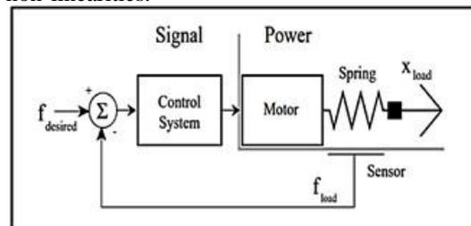
Fig .3 Series elastic actuator block diagram.[25]
