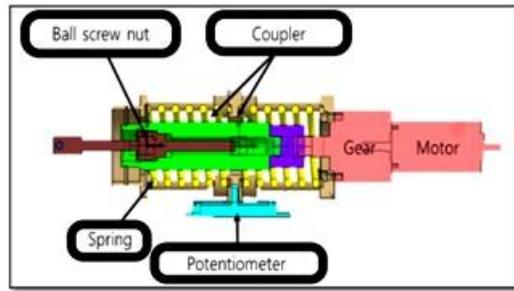
Fig.1 The series elastic actuator Configuration [25].
