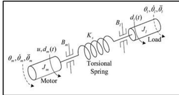
Fig.10 The SEA dynamic process's schematic diagram.[28]
