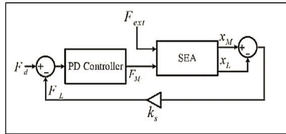
**Fig.14** Block diagram of SEA controller.[30]
