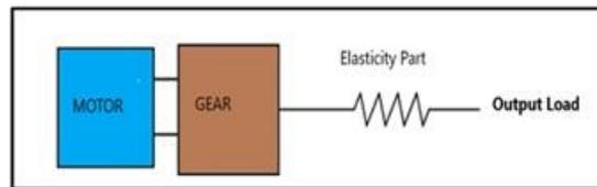
Fig.2 Series elastic actuator model [25].
