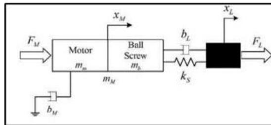
Fig.13 The translational motion of the SEA according to the dynamic model.[30]
