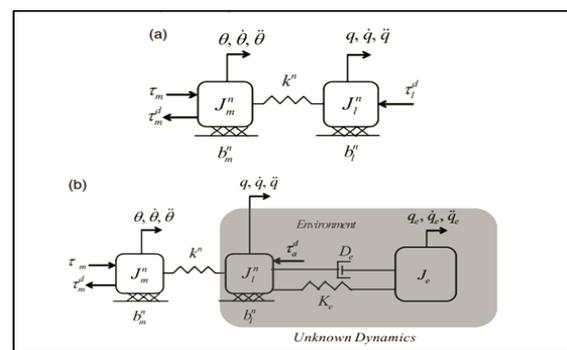
**Fig.15** Dynamic models of SEA. (a) Free motion. (b) environment interaction.[31]
