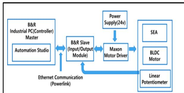
Fig.5 Control system for SEA hardware configuration [25]
