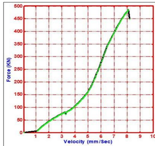
Fig. 9. The propriospinal between extrusion speed and extrusion force.
