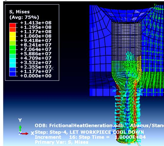
Fig. 7. Contours plot of equivalent Von Mises stresses.
