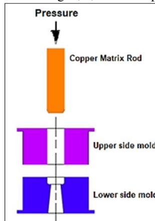
Fig. 2. Alignment of parts with billet.
