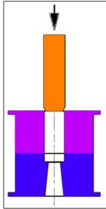
Fig. 3. Applying extrusion force.
