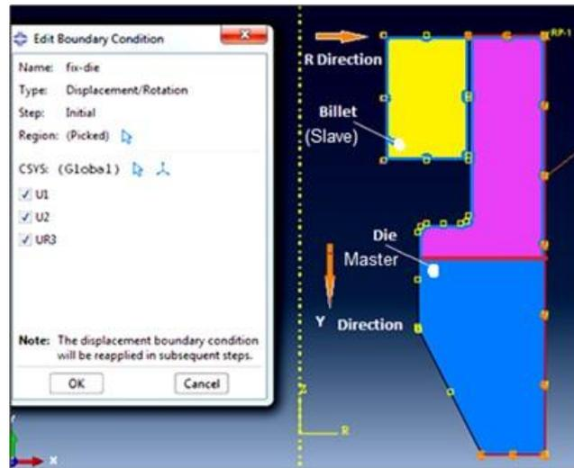
Fig. 6. Constrain and boundary conditions relationship.
