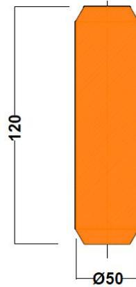
Fig. 1. The composite rod with all dimensions.
