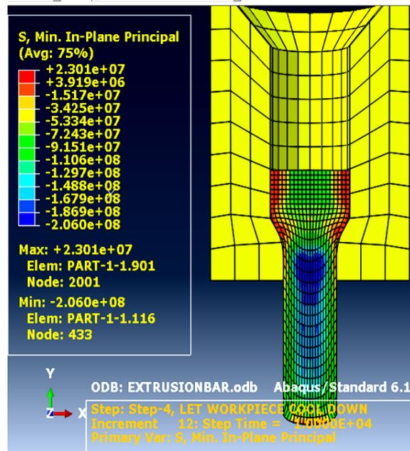
Fig. 8. The contour plot of the principal stresses in plane.
