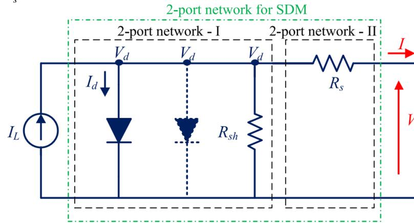
Figure 3. Equivalent circuit of single diode model (SDM)/double diode model (DDM) with two 2 port networks.
