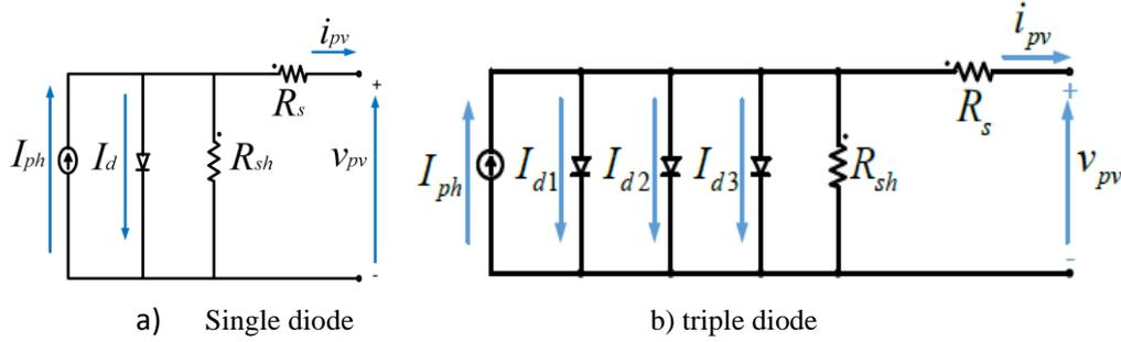
Figure 1. PV panel circuit approach model
