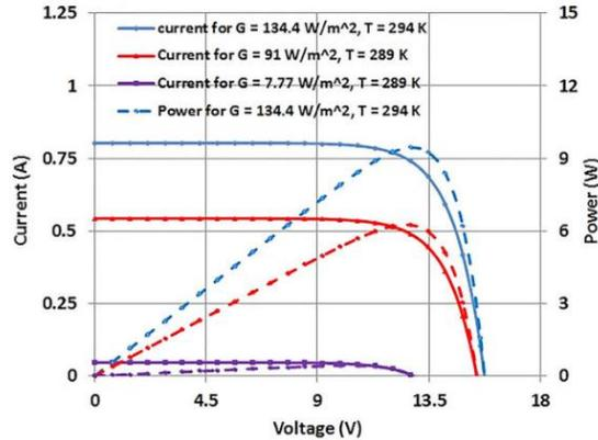
Figure 2. Manufacturer's data PV characteristic curve at standard test conditions (STC).
