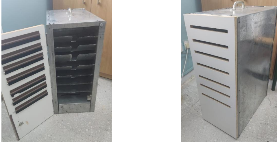
Figure 1: Front-end design and the internal paper tray for the prototype.
