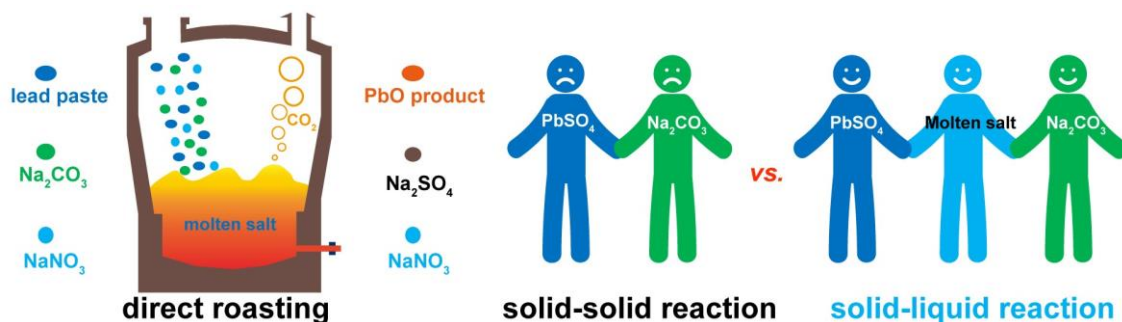
Scheme 1 Schematic diagram of flow chart of the molten nitrate salt assisted approach for direct smelting of spent lead paste
