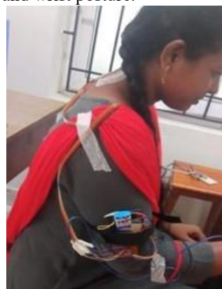
Figure .9. Prototype with flex sensor Placed in the wrist
