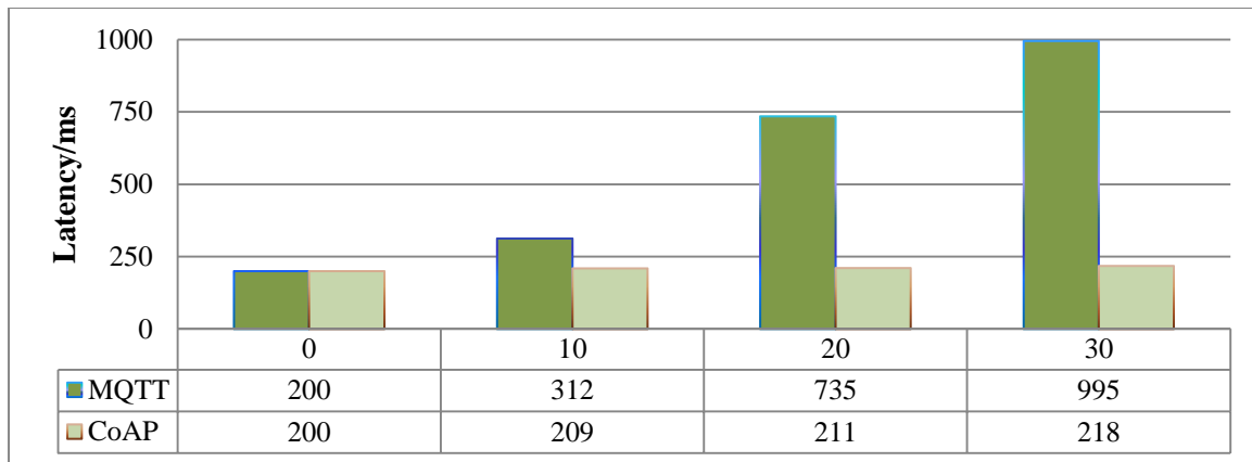
Figure. 8 Analysis of protocols in terms of packet loss and latency.
