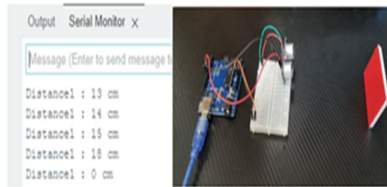
Fig. 2. Ultrasonic sensor test result
