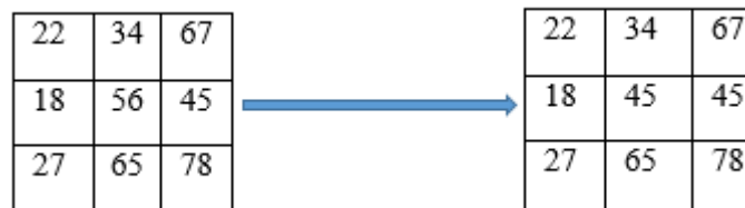
Figure 2. Original values of 3 \times 3 window 3 \times 3 window after applying a median purifier.
