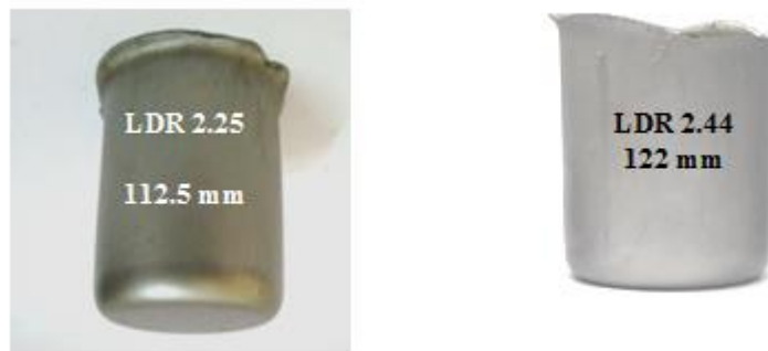
Figure 6. Successfully formed cup of AISI 304 with maximum LDR a) Isothermal Forming (a) Non- Isothermal Forming
