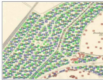
Fig. 1. A subset of the map is subjected to tree template matching with a threshold of 0.6; each box indicates a match, and the color of the box indicates which template it matches with
