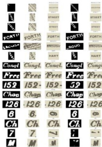
Fig. 16. The text masks as predicted by the trained UNet model are displayed in the fourth column. The fifth column displays the predicted images following orientation adjustments and noise reduction using the updated predicted masks in conjunction with the updated predicted text generated by Pytesseract
