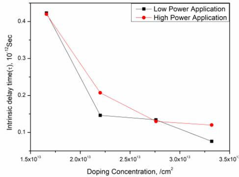
Fig. 13. Calculated Intrinsic delay time ( $\tau$ ) plot as a function of different doping concentrations in DG JLFET device for HP and HD applications. Red dashed lines represent the delay time for HP application and black dashed line for HD application.
