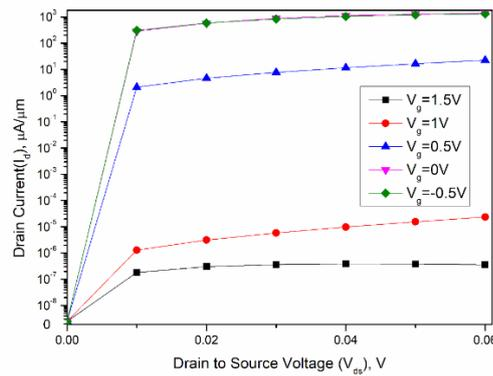
Fig. 3. Comparative drain current plot as a function of drain-to-source voltages ( $V_{ds}$ ) for various doping concentrations ranging between  $(1.66 - 3.32) \times 10^{13} \text{ cm}^{-2}$  with a variation of gate to source voltage ( $V_{gs}$ )
