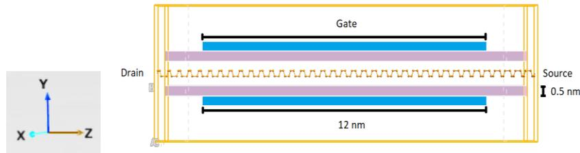
Fig. 1. The schematic diagram of lateral JLFET
