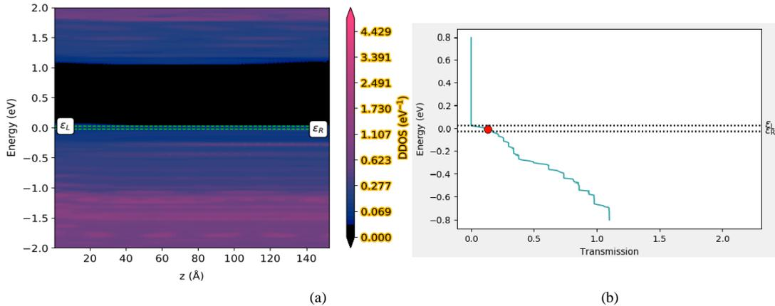
Fig. 11. Projected local density state (PLDOS) along source to drain and the corresponding transmission spectra of on-state for the DG-JLFET with gate length  $L_g = 12\text{nm}$ . The green/black dash line indicates the source to drain tunneling window  $V_{ds} = 0.05\text{V}$  corresponding to right and left Fermi levels of the electrodes.
