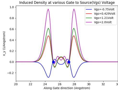
Fig. 9. Variation of depletion charge density ( $n_y$ ) for  $2.20 \times 10^{13} \text{ cm}^{-2}$  p-type doping as a function of gate-to-source voltages along gate direction ( $y$ ) in DG JLFET device.
