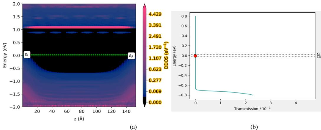
Fig. 10. Projected local density state (PLDOS) along source to drain and the corresponding transmission spectra of OFF-state for the DG-JLFET with gate length  $L_g = 12\text{nm}$ . The green/black dash line indicates the source to drain tunneling window  $V_{ds} = 0.05\text{V}$  corresponding to right and left Fermi levels of the electrodes.
