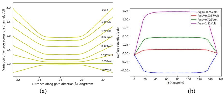
Fig. 8. (a) Variation of voltage ( $v-y$ ) along gate direction ( $y$ ) direction for different applied gate biases (b) Variation of electrostatic potentials for  $2.20 \times 10^{13} \text{ cm}^{-2}$  p-type doping as a function of gate-to-source voltages along the channel direction ( $z$ ) in DG JLFET device.
