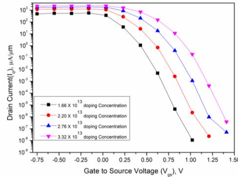
Fig. 2. Comparative drain current plot for different doping levels as a function of gate-to-source voltages ranging between  $(1.66 - 3.32) \times 10^{13} \text{ cm}^{-2}$  with a drain to source voltage ( $V_{ds}$ ) = 0.05 Volt
