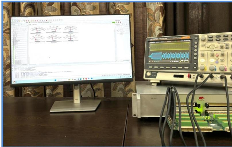
Figure 4. The real-time simulation test setup, utilizing the Typhoon HIL604 real-time simulator.
