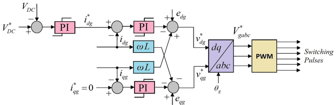
Fig.3. The voltage-oriented control for the LSC.
