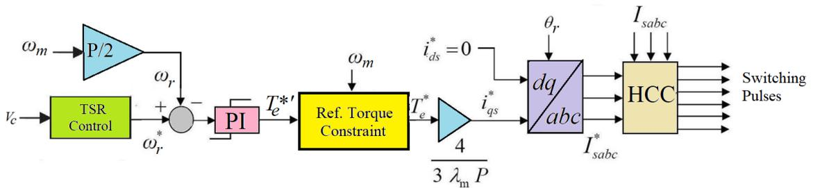
Fig.2. The proposed control for the generator-side VSC.
