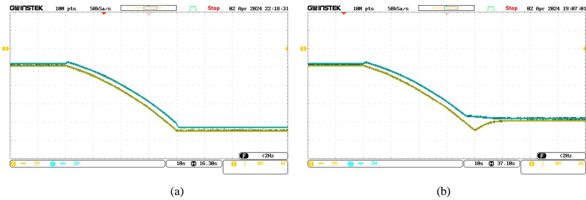
Fig. 6. Real-time results under (a) URTM and (b) CRTM—Ch.1: MCT power (400 kW per div); Ch.2: Generated power (400 kW per div).
