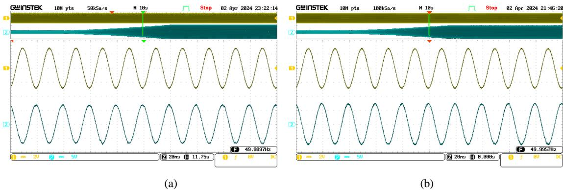
Fig. 10. Real-time results (zoomed view) under (a) URTM and (b) CRTM demonstrating unity power factor operation—Ch.1: Phase-a grid voltage (400 V per div); Ch.2: Phase-a grid current (1000 A per div).
