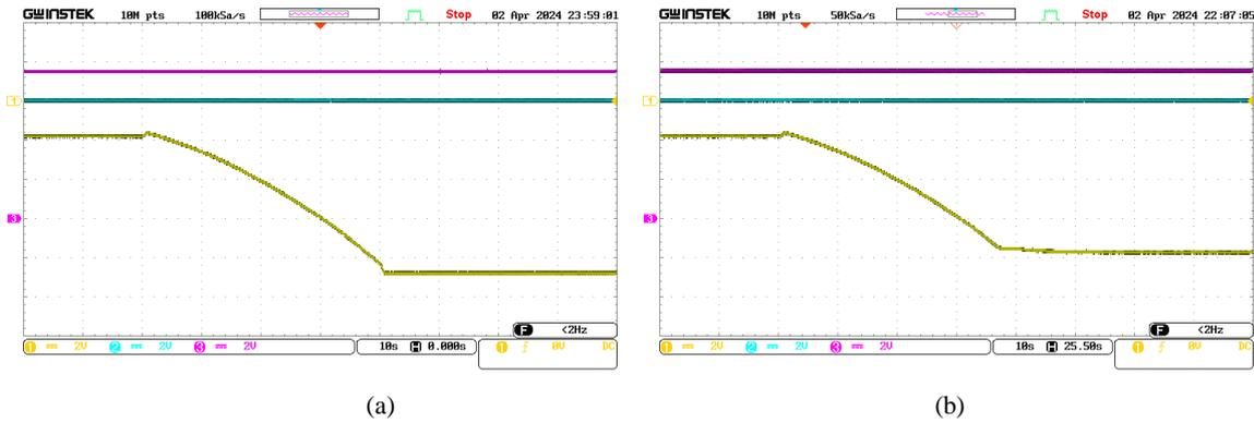
Fig. 9. Real-time results under (a) URTM and (b) CRTM—Ch.1: Grid-side active power (400 kW per div); Ch.2: grid-side reactive power (400 kVAR per div); Ch.3: DC-link voltage (400 V per div).
