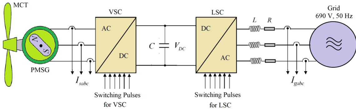
Fig.1. The proposed grid-tied PMSG-based MCTS.
