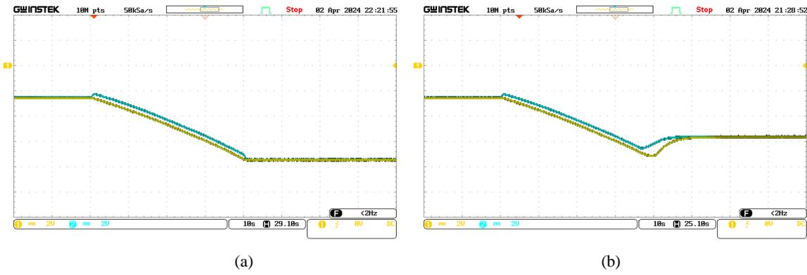
Fig. 7. Real-time results under (a) URTM and (b) CRTM—Ch.1: MCT torque (200 kN per div); Ch.2: Generator torque (200 kN per div).
