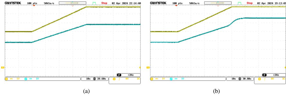
Fig. 5. Real-time results under (a) URTM and (b) CRTM—Ch.1: Marine current speed (0.5 m/s per div); Ch.2: Generator rotational speed (0.5 rad/s per div).
