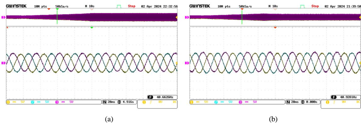
Fig. 8. Real-time results (zoomed view) under (a) URTM and (b) CRTM—Ch.1: Phase-a generator current (2000 A per div); Ch.2: Phase-b generator current (2000 A per div); Ch.3: Phase-c generator current (2000 A per div).
