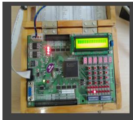
Fig 14. Digital DTC implementation on a Xilinx Spartan-3 FPGA board
