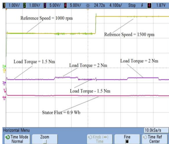
Fig. 17. Speed and electromagnetic torque response for various reference speeds and load torques
