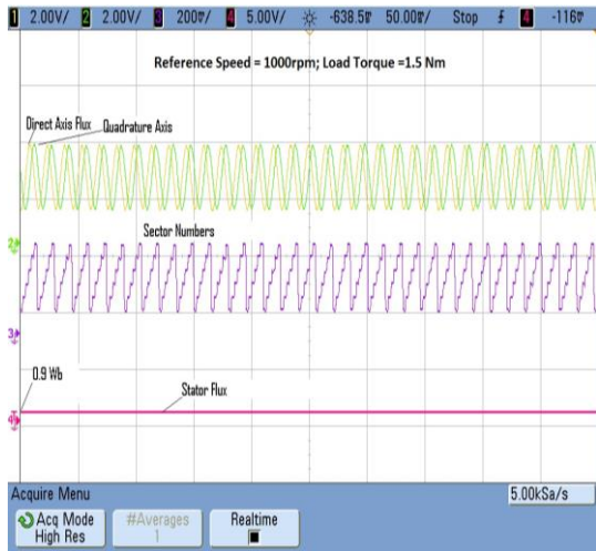
Fig. 15. Direct and Quadrature axis flux response, Stator flux response and sector numbers for reference speed of 1000 rpm and load torque = 1.5 Nm
