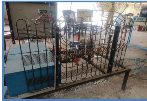
Fig-2 Fins Type Condenser Arrangement
