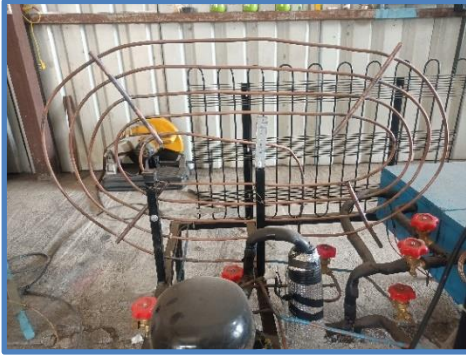
Fig-1 Spiral Condenser Arrangement
