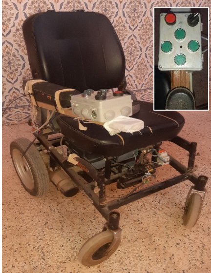
Fig 7. Modified Electric wheelchair (without joystick)
