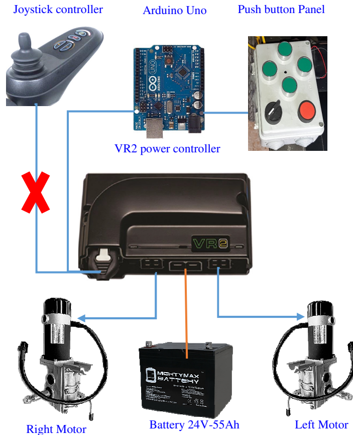
Fig. 2. Schematic diagram of the developed system
