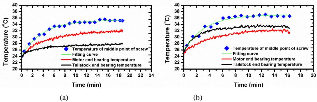
Figure 4. Temperatures of the middle interval of the Y-axis screw stroke and bearings at both ends under different installation methods: (a) state 1, (b) state 2.
