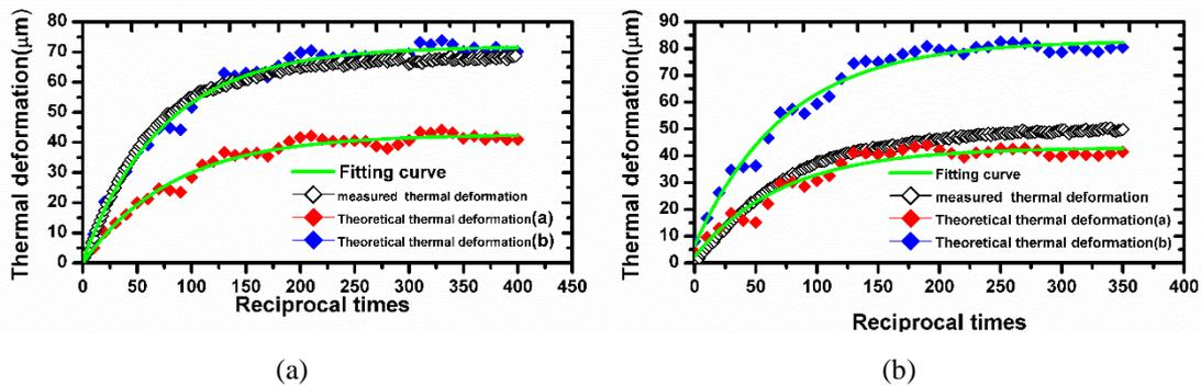
**Figure 9.** Thermal deformation in the Y-axis stroke section: (a) state 1, (b) state 2.
