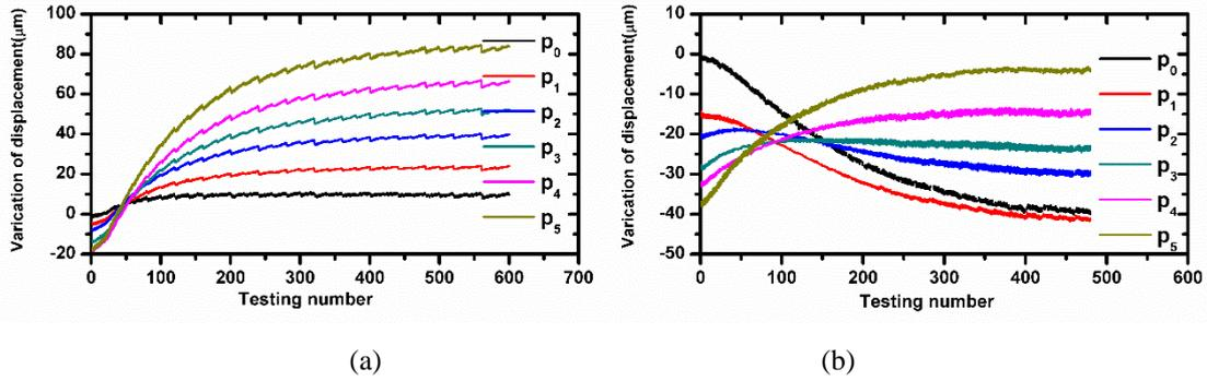
Figure 6. Thermal displacement of the X-axis stroke: (a) state 1, (b) state 2.
