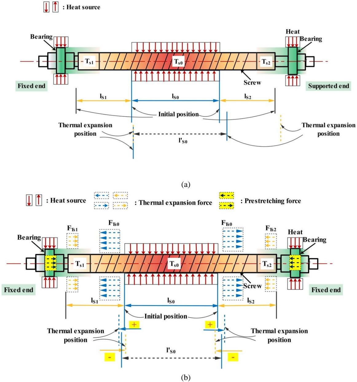
**Figure 1.** Thermal expansion for two installation modes: (a) one end fixed and the other supported (state 1), (b) both ends fixed (state 2).
