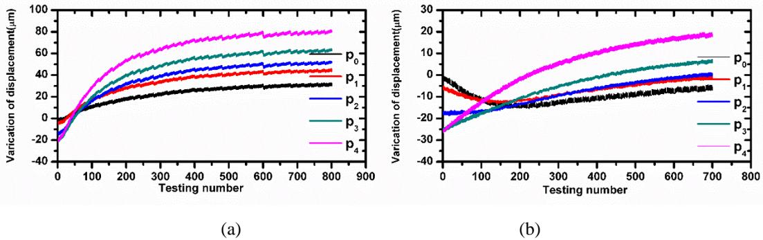
Figure 7. Thermal displacement of the Y-axis stroke: (a) state 1, (b) state 2.
