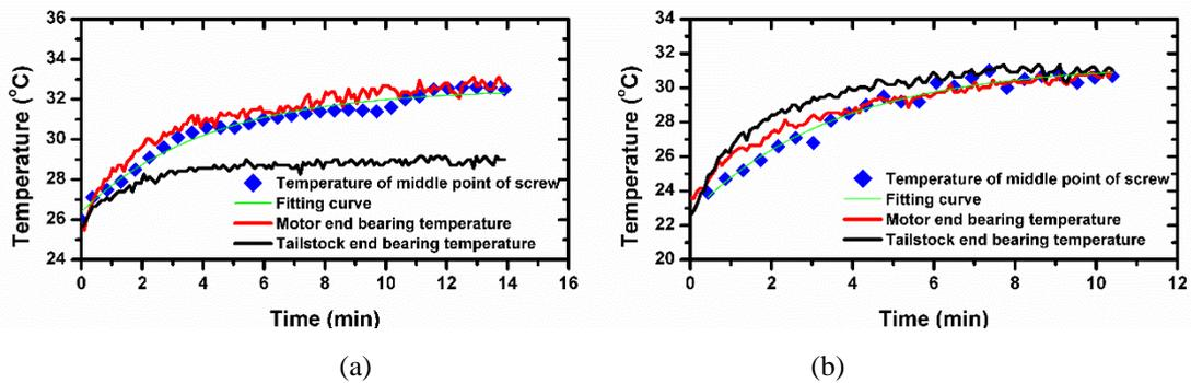
Figure 3. Temperatures of the middle interval of the X-axis screw stroke and bearings at both ends under different installation methods: (a) state 1, (b) state 2.
