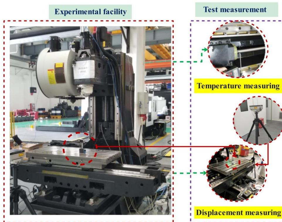
**Figure 2.** Test device and test diagram.
