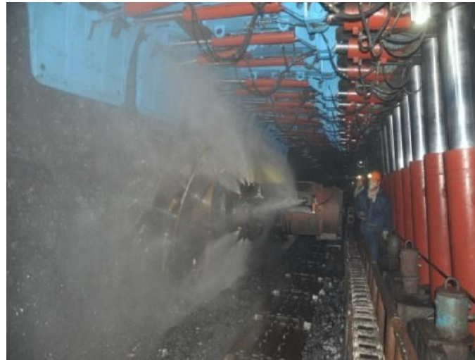
Figure 1: Internal and external spray used to coal dust [1]
