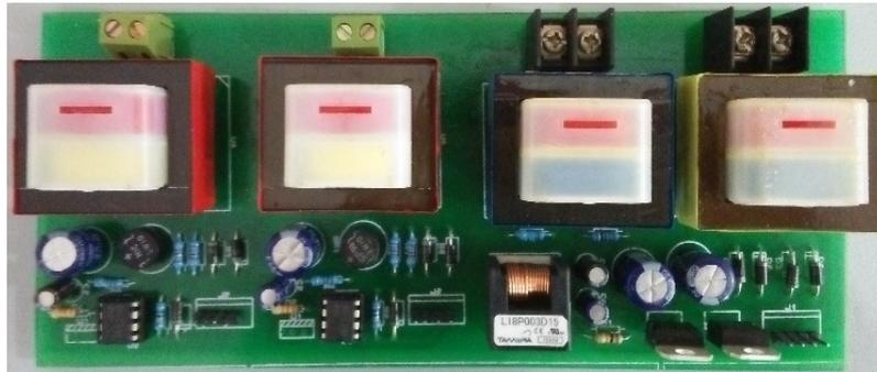
Figure.11: Data acquisition card for grid voltage and current sensing
