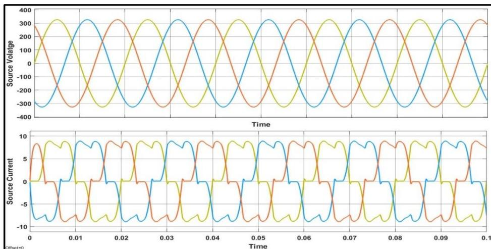
Fig.5. Source current and Voltage Waveforms Without SAPF
