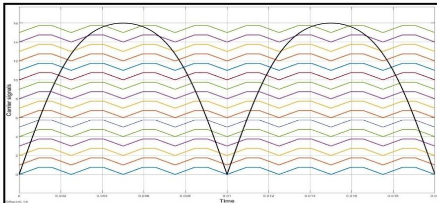
Fig.2. Hybrid Pulse Width Modulation
