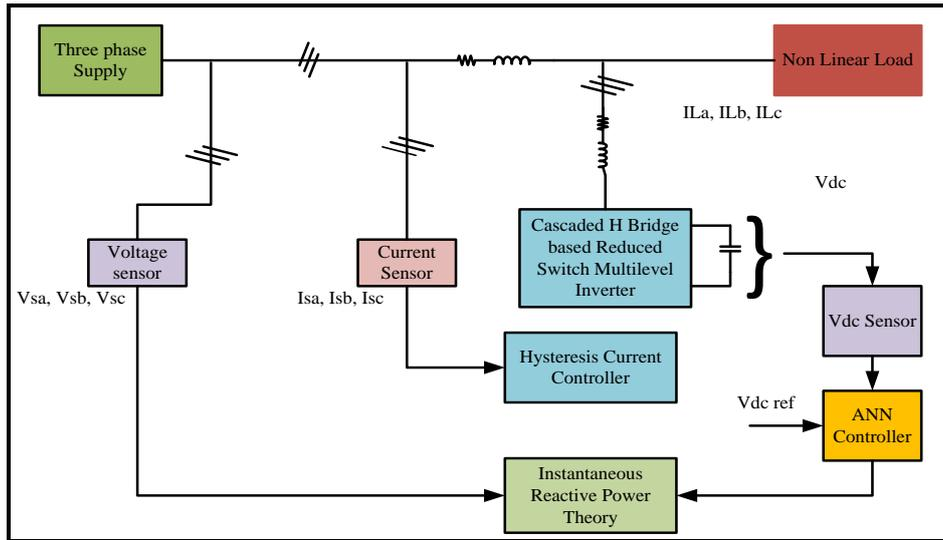
Fig.3. Block Diagram of RSMLI-SAF based p-q Theory
