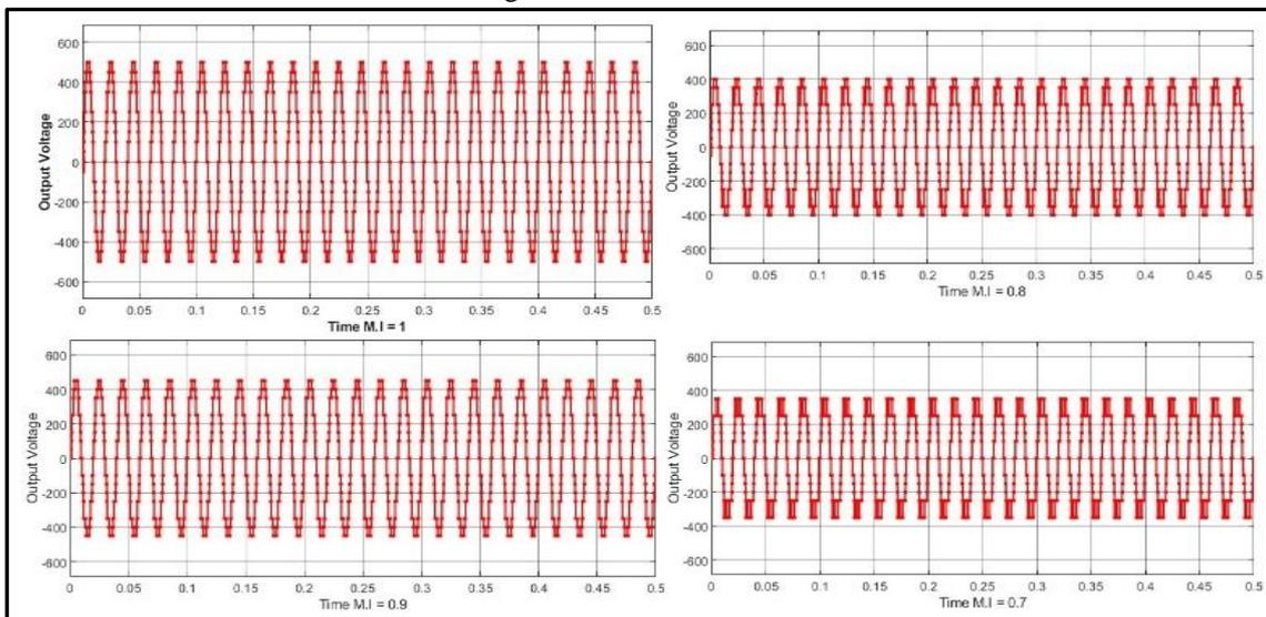
Fig.7. Output Voltage Waveforms for Various MI's
