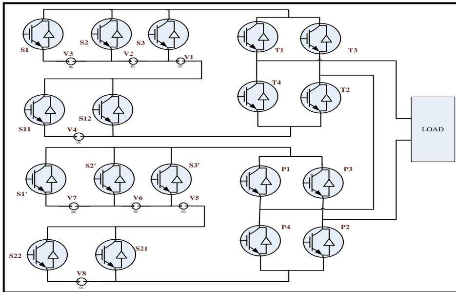
Fig.1. Proposed Seventeen level RSMLI Topology
