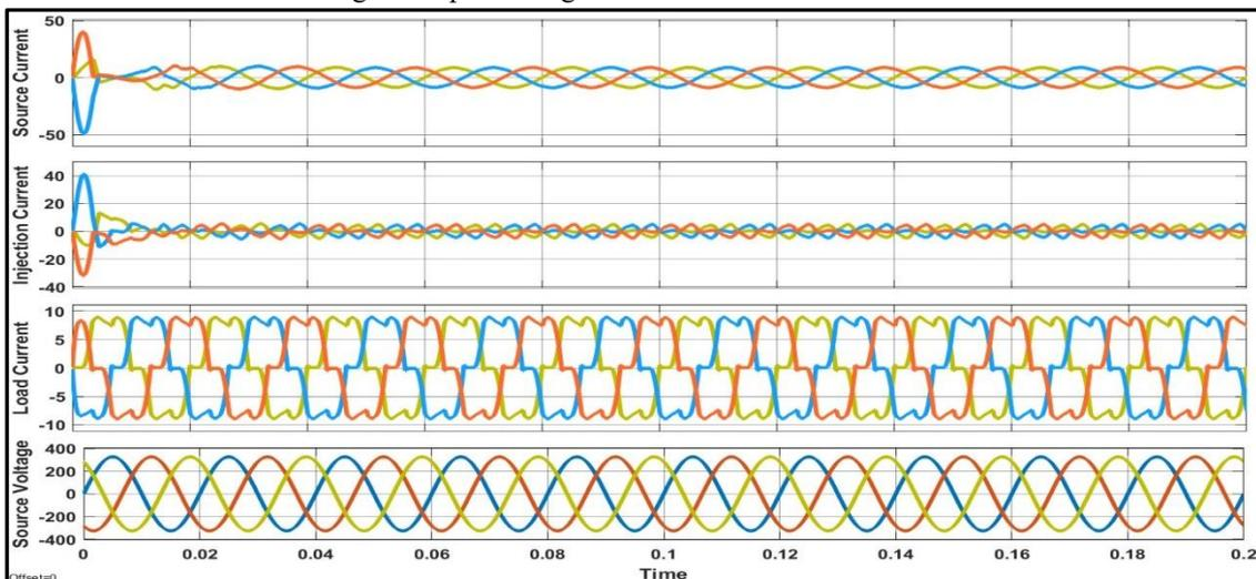
Fig.8. Source current Waveform with PI Controller
